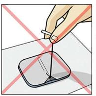
• Do not remove Electrodes by pulling the leadwire.
