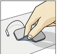
• Remove Electrodes by lifting the edge.
